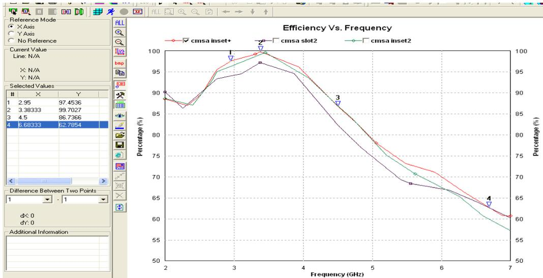
Fig. 8. Efficiency vs frequency comparative study of a circular patch with /without slots
