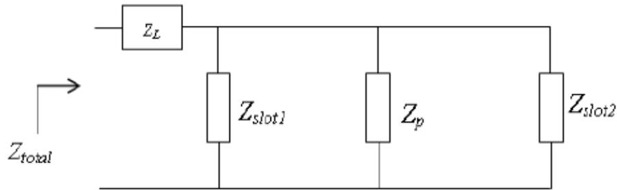
Fig. 4. Equivalent circuit of Asymmetric Cross slot Loaded L strip
