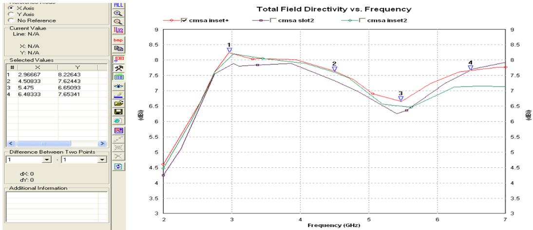
Fig. 6. Directivity vs frequency comparative study of a circular patch with /without slots
