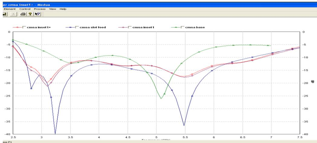
Fig. 5. Reflection Coefficient vs frequency comparative study of a circular patch with/without slots
