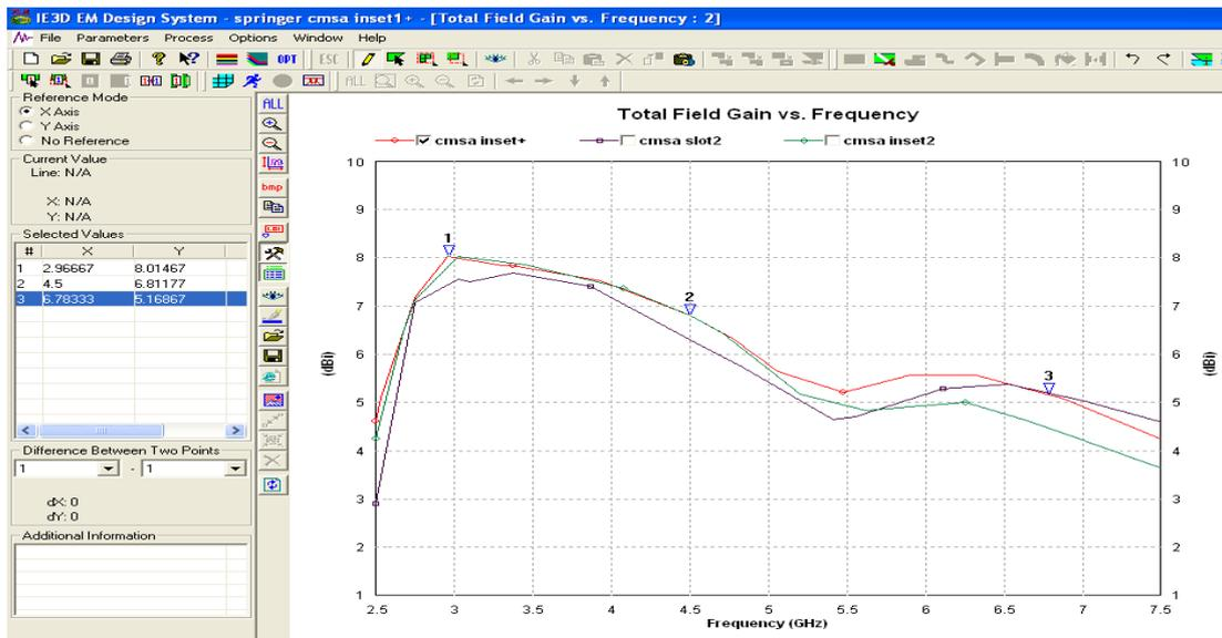
Fig. 7. Gain vs frequency comparative study of a circular patch with /without slots
