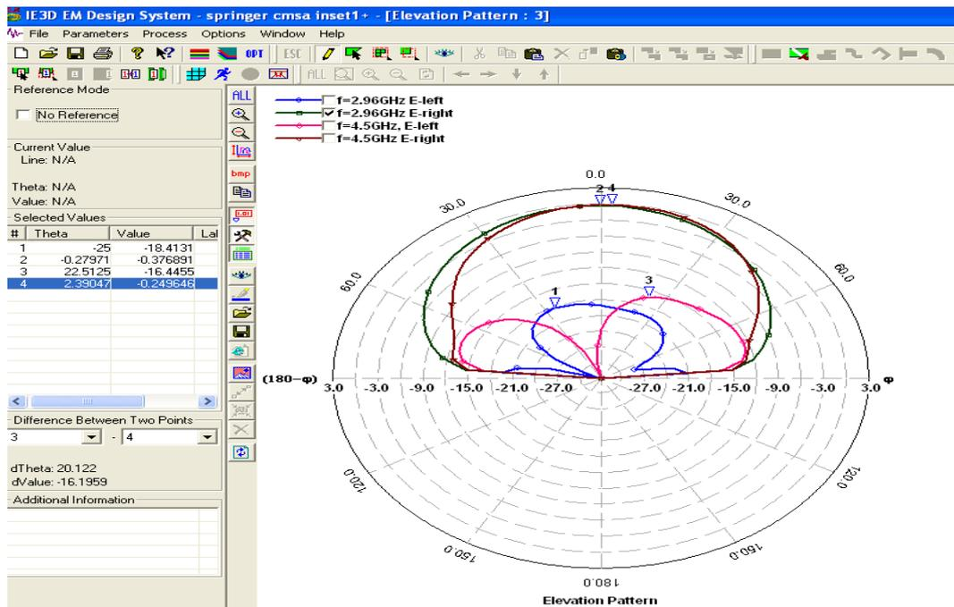
Fig. 12. Elevation pattern for circular polarisation (RHCP and LHCP) for CMSA inset +
