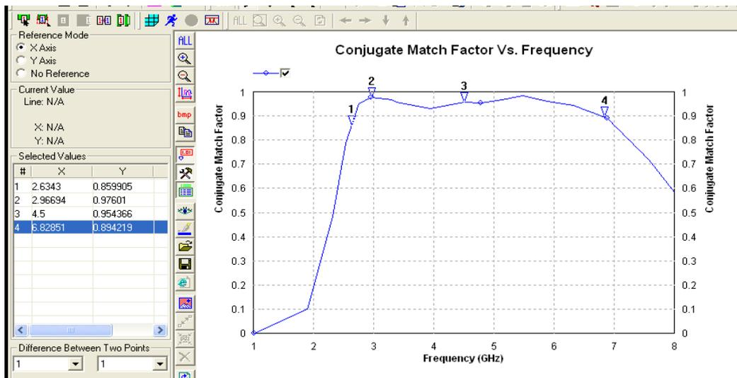
Figure 9 Conjugate Impedance matching vs frequency for cmsa inset+
