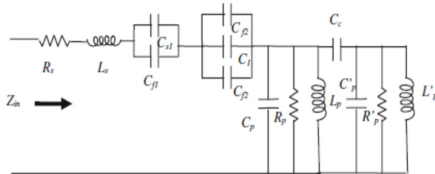
**Fig.3 Equivalent circuit of circular patch with any of slots**
