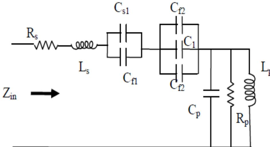
Fig.2 equivalent circuit of circular patch
