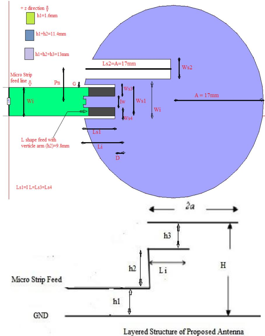
Fig. 1. Geometry of parallel slots loaded L-strip fed proximity coupled circular micro strip antenna (a) Top view (b) Side view
